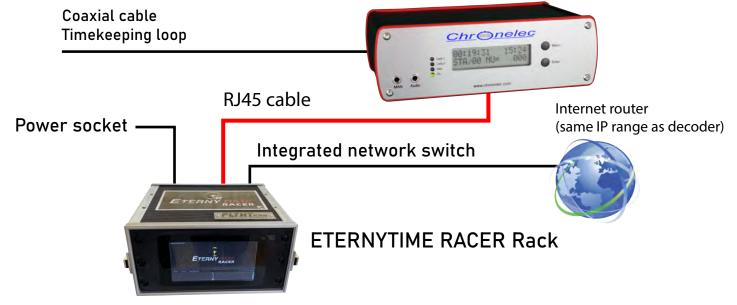
The ETERNYTIME Racer server uses DHCP to get it's IP automatically. Internet connexion and timekeeping decoder should be on same IP range. ex. Internet router: 192.168.0.1 and decoder 192.168.0.10
